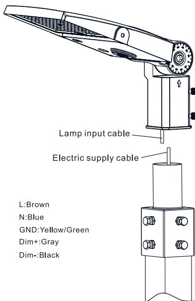
6. The wires are hidden inside the lamp post, and the lamp is fixed to the lamp post with screws. Adjust the light output angle of the lamp.
