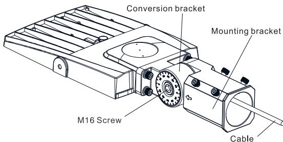
4. Install the adapter bracket onto the lamp post using M10 screws.
