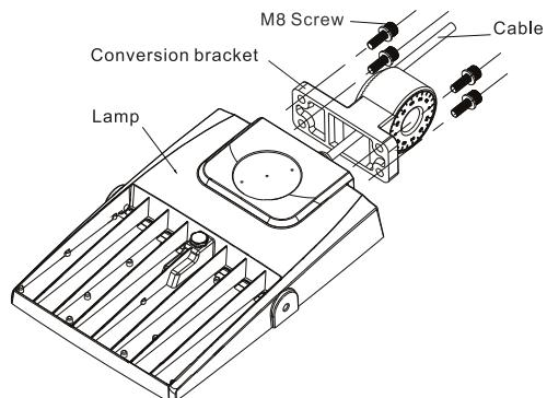
3. The cable passes through the mounting bracket; The mounting bracket and conversion bracket are fixed together with M16 screws.
