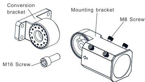
2. The cable passes through the conversion bracket and is fixed conversion bracket to the lamp with M8 screws.
